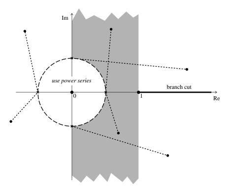
Figure 5.14.1. Complex plane showing the singular points of the hypergeometric function, its branch cut, and some integration paths from the circle |z|=1/2 (where the power series converges rapidly) to other points in the plane.
