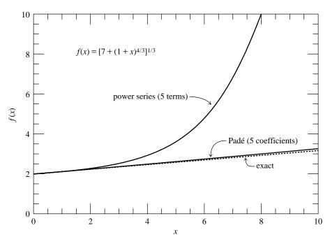
Figure 5.12.1. The five-term power series expansion and the derived five-coefficient Padé approximant for a sample function f(x). The full power series converges only for x < 1. Note that the Padé approximant maintains accuracy far outside the radius of convergence of the series.
