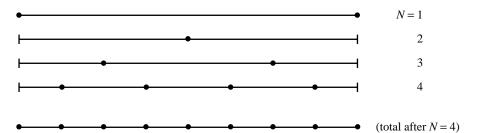
Figure 4.2.1. Sequential calls to the routine trapzd incorporate the information from previous calls and evaluate the integrand only at those new points necessary to refine the grid. The bottom line shows the totality of function evaluations after the fourth call. The routine qsimp, by weighting the intermediate results, transforms the trapezoid rule into Simpson's rule with essentially no additional overhead.
