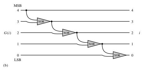
Figure 20.2.1. Single-bit operations for calculating the Gray code G(i) from i (a), or the inverse (b). LSB and MSB indicate the least and most significant bits, respectively. XOR denotes exclusive-or.
