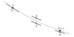
Figure 16.1.3. Fourth-order Runge-Kutta method. In each step the derivative is evaluated four times: once at the initial point, twice at trial midpoints, and once at a trial endpoint. From these derivatives the final function value (shown as a filled dot) is calculated. (See text for details.)
