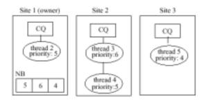
Threads waiting in the CQs at three sites. Site 1 is the owner site of the monitor It keept the valid notification board. If the current running thread at Site 1 executes *notify*, Thread 3 is notified. If *notify-all* is executed, all the waiting threads are notified.
